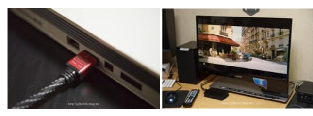
The image on the left is PS3 for blu-ray movies and games. I connected the PS3 and 3D TV with HDMI cable. HDMI cable is capable of transmitting both the video and audio at the same time. Therefore 3D TV takes charge of the final transmission to LA-200. Right now, the 3D TV is connected to LA-200 using Optical cable by two kinds of audio input; PC1's analog input and PS3's HDMI.
