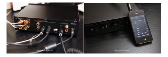
When you look at the back panel of LA-200, you can see I have 3DTV connected to D3 (Optical digital), PC2 to USB, iPhone 4 to iPod (Analog mini stereo). As for now, only analog transmission is possible for iPhone 4 or iPod.
